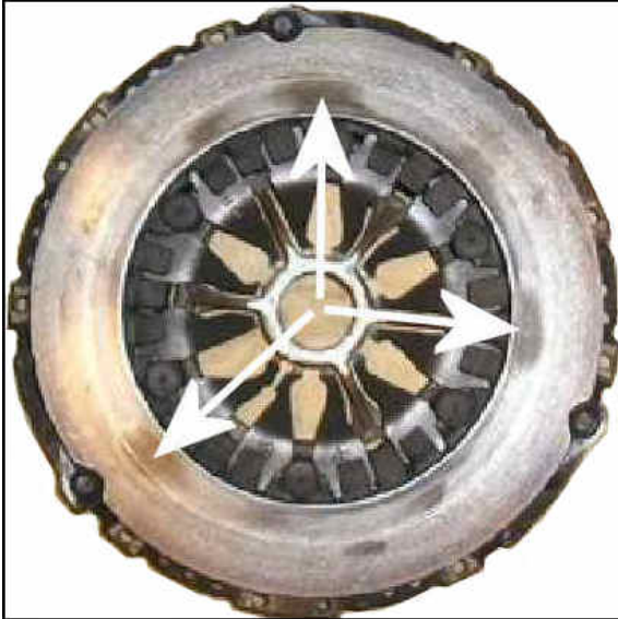
Heat spots on pressure plate contact surface.
