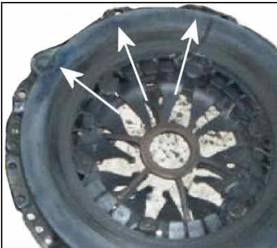
Blued heat spots on pressure plate contact surface.
