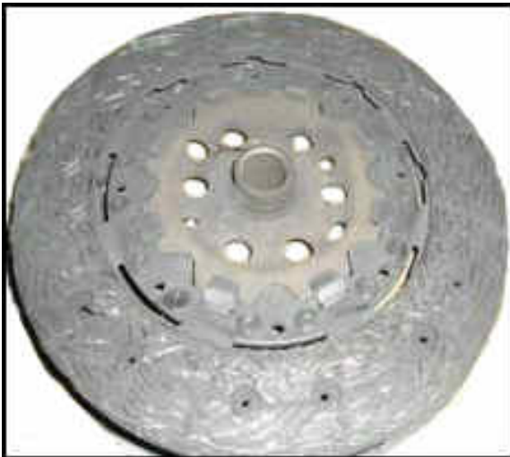
Clutch plate material burnt.
