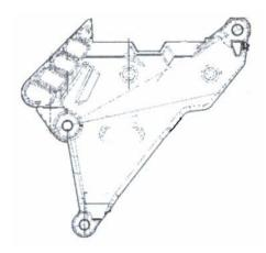
Verify that the support being replaced is old style support Part No. 03G199207F.
