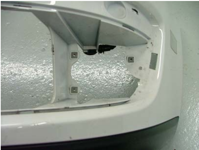
Speed clip inserts installed.
